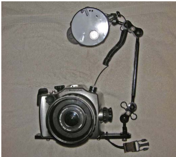
A polycarbonate housing, assembled with a camera tray, lens port, and external strobe.
