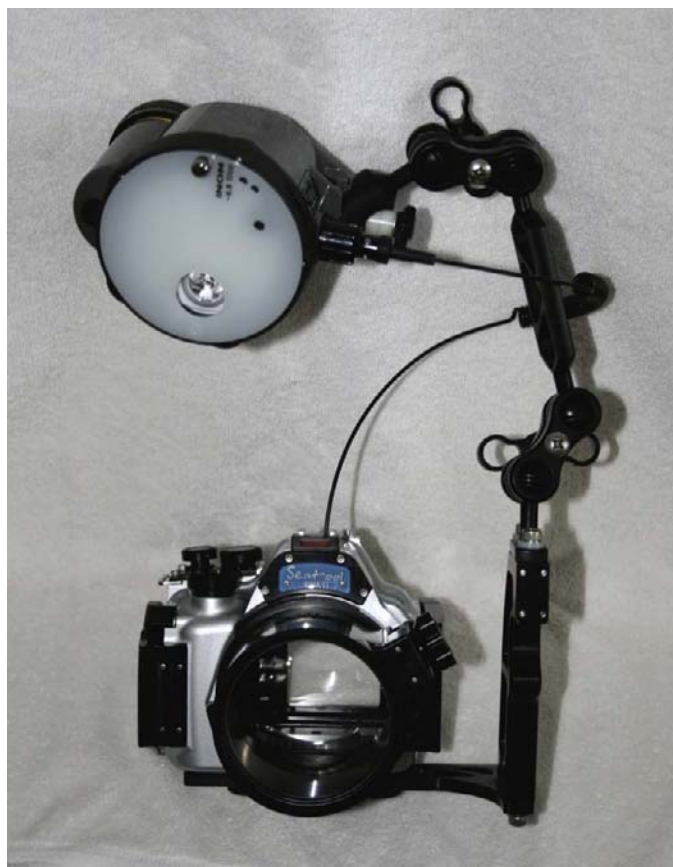
A digital single lens reflex (dSLR) with housing, port, camera tray, handle, clamp, strobe arm, strobe head adapter and strobe, diffuser, and a fiber optic array.
