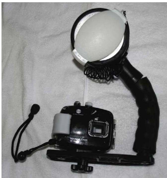
The strobe is slaved to the camera.
